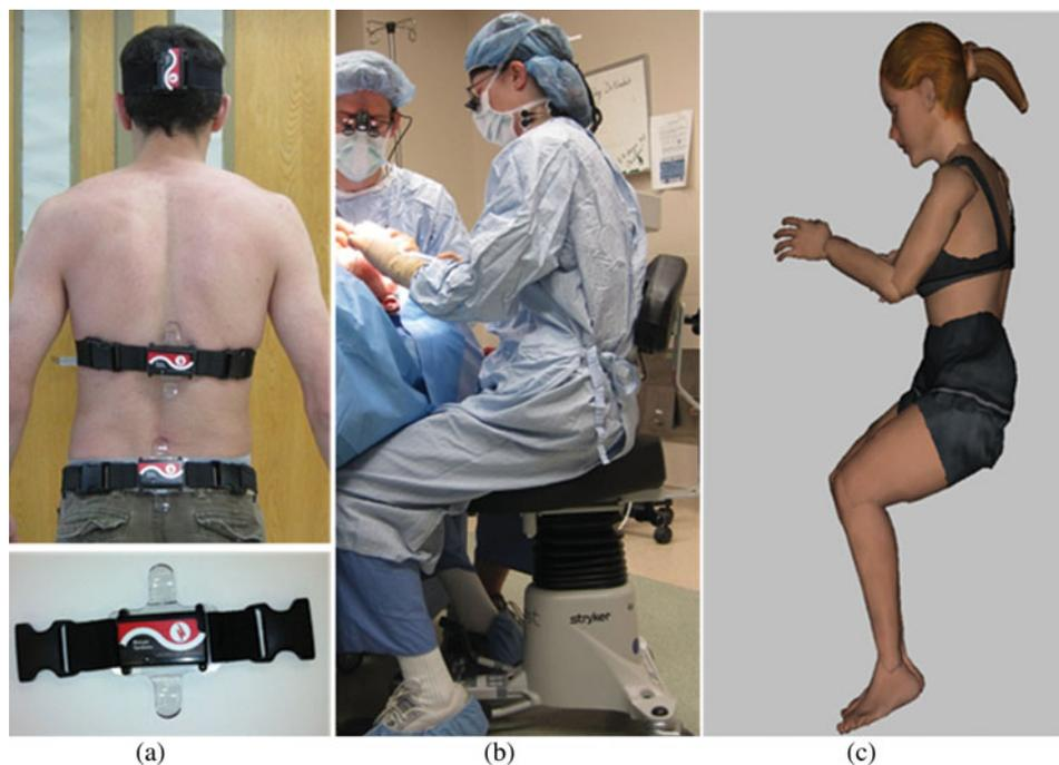
**FIGURE 1** (a) FAB sensors and their locations for recording head-neck kinematics, (b) a surgeon performing surgery, and (c) real-time humanoid displayed by FAB system. To generate this humanoid, all 13 FAB sensors were used during pilot data collection (color figure available online).
