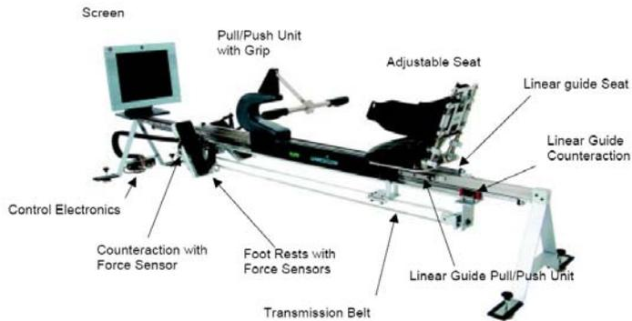
Figure 3 Endurance Trainer - example countermeasure device
