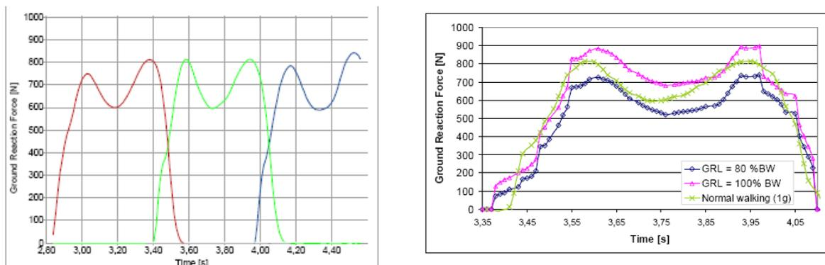
Figure 11 Ground reaction forces: on the left from 1g walking (red: right foot contact, green: left foot contact, blue right foot contact) and on the right the harness induced 0g walking (one foot contact shown only). The GRL indicates the percentage of body weight used.
