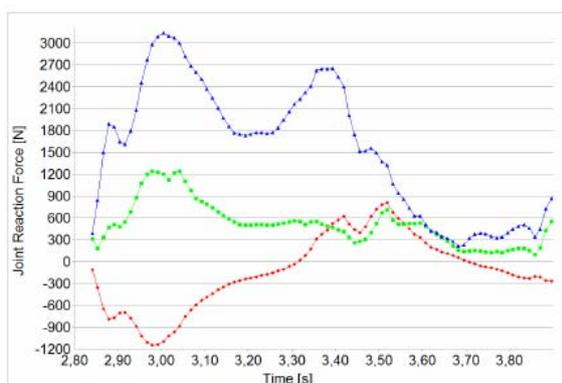
Figure 9 Hip Reaction Forces during normal 1g walking. The different curves refer to the force components in the global coordinate system: inferior-superior (blue), anterior-posterior (red) and medial-lateral (green).
