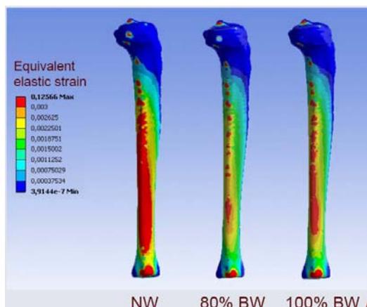
Figure 12 result of bone strain analysis. NW is representing 1g condition, 80% and 100% BW are representing 0g conditions with the harness (80% and 100% of the body weight)
