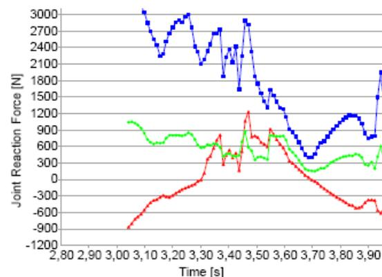
Figure 10 Hip Reaction Forces during 100%Body Weight (BW) 0g walking
